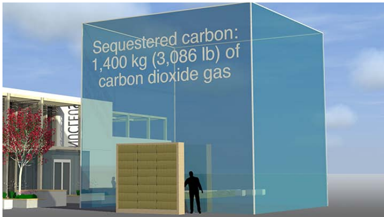
A typical 3m x 3.2m ModCell panel sequesters 1,400kg of CO 2
