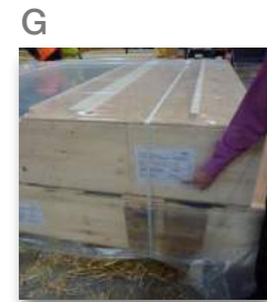
G Panels are closed and uniquely marked as part of ISO 9001 2017 quality management system
