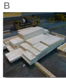
B Engineered timber arrives 'flat packed' to flying factory minimising the embodied carbon resulting from transportation.
